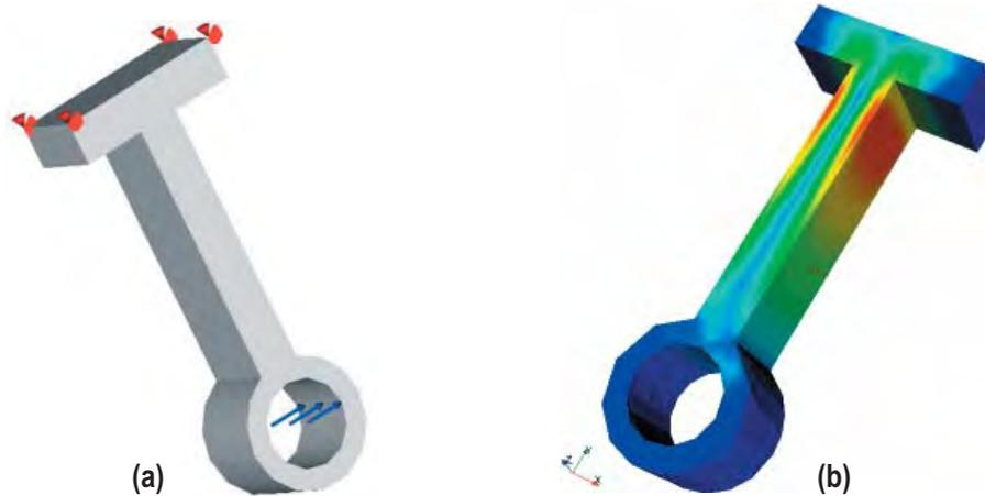
Using the theoretical concepts presented in this article, an application named *Provolution* was developed under PRO/ENGINEER's API, PRO/TOOLKIT. This application provides the user with a friendship interface to solve 3-D linear elastic problems using FG-FEA, and perform shape and dimensions optimization by means of Evolution Strategies. An example of a model optimized using *Provolution* is presented in Figure 5 and Figure 6.
